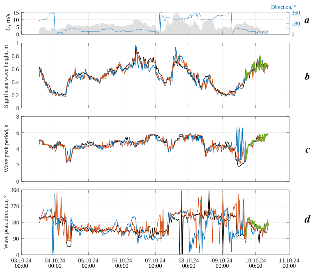
Fig. 3. Wind speed and direction ( a ) during the experiment, time series of wave parameters estimated from measurements of wave gauge (black) and Buoys 1 (blue), 2 (orange), 3 (green): b – significant wave height; c – spectral peak wave period; d – spectral peak wave direction
