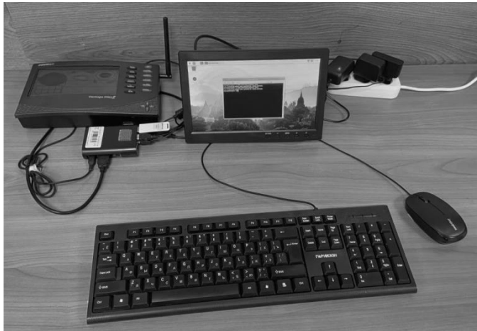
Fig. 1. The appearance of the workplace for automated measurements, transmission and storage of the weather station Davis Vantage Pro 2 data using a Raspberry Pi B+
