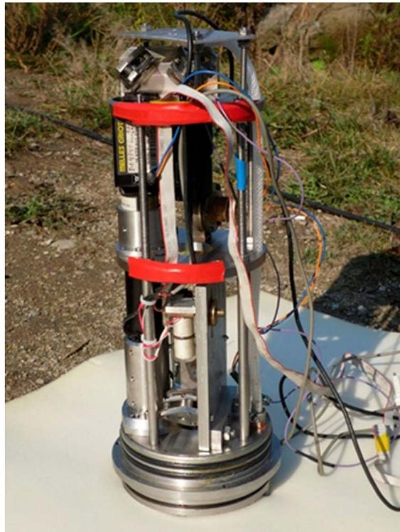
**Fig. 1.** Supersensitive detector of hydrosphere pressure variations, inside
